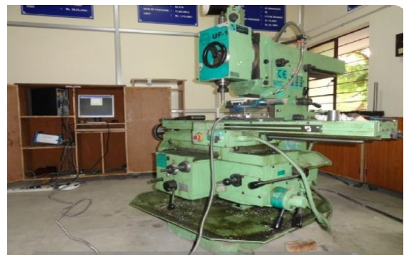
Fig 1: End milling operations were carried out in a BHARAT FRITZ WERNER BF-1 universal milling machine with 2.2 kW motor capacity.
