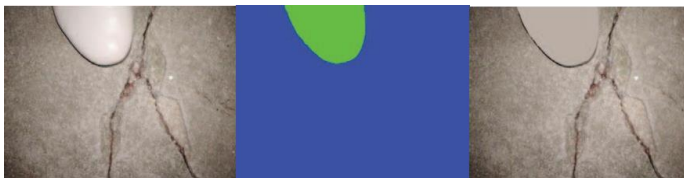
(a) Original image (b) segmentation result (c) filled image Fig.2 Pretreatment effect
