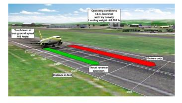
Figure 3. Necessary of cascade thrust reverser
