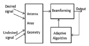
Figure 1. Block diagram of Smart antenna system
