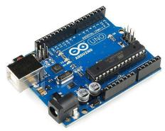
Figure 3. Arduino ATMEGA 328 kit
