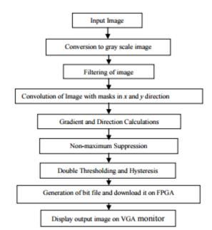
Figure. 2 Flow of Canny Edge Detection Algorithm
