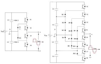
**Figure 1.** One phase leg of DCMLI (a) 3 level; (b) 5 level
