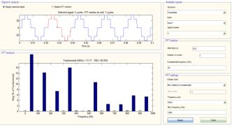
**Figure 5(a)** THD analysis of 5 level DCMLI with R load (THD = 31.13%)
