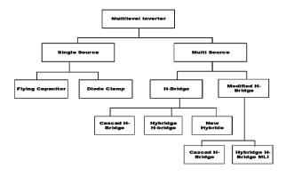
Voltage Source Multilevel Inverters has been broadly classified in to two parts depending upon the number of voltage sources as shown below:
