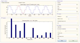
**Figure 5(b)** THD analysis of 5 level FCMLI with R load (THD = 28.50%)
