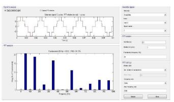
**Figure 9.** THD analysis of 5 level DCMLI with R load (THD = 31.13%)
