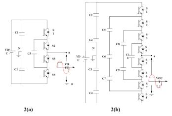
Figure 3. One phase leg of CHB (a) 3 level; (b) 5 level
