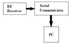
Figure 1. Block Diagram of Server Section
