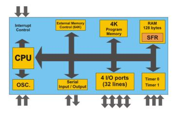
Figure 3. Microcontroller Internal Structure
