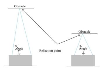
**Figure 1.** Reflection of light making different angles depending on the distance of the reflecting object.
