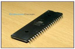
Figure 2. Atmega 16 Microcontroller
