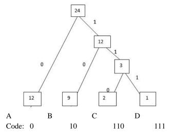
No. bits required for uncompressed data: 24 \* 8 =192 bytes No. bits required for compressed data : 9 \* 8 = 72 bytes
