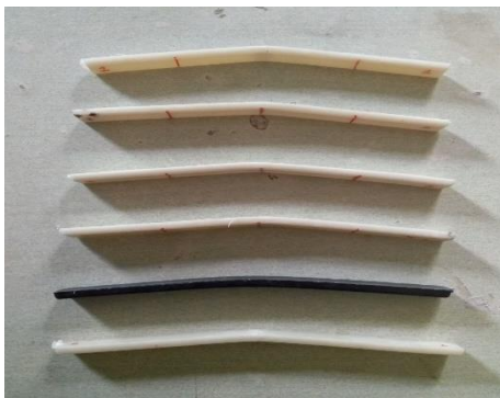
Fig 6: Flexural test specimens after testing
