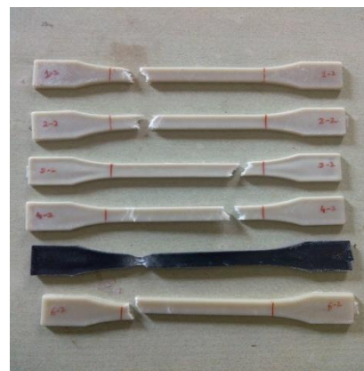
Fig 4: Tensile test specimens after testing
