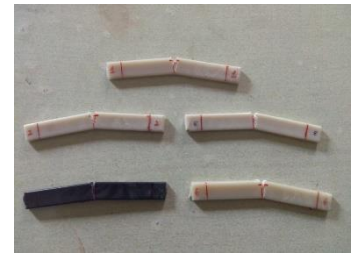
Fig (9): Izod impact test specimen after testing
