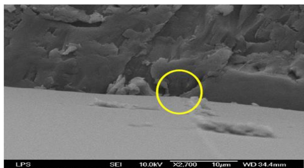
Collapsed microchannel after thermo-mechanical deformation at 70% strain
