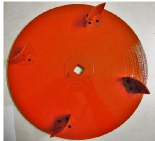
Figure 5: (a) Rotating disc apparatus 3D modelling and (b) disc with CFT blade test specimens Adopted from Shrestha [30]
