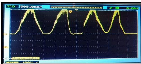
Fig 3.6: Voltage induced in a very fast running
