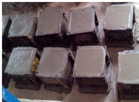
Sampling of concrete
