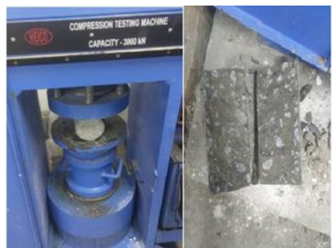
Figure 4.2 : Split tensile test of concrete
