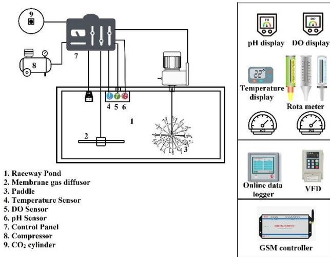
**Figure 1:** A graphical representation of the 1500 litre open raceway pond, including the control panel and CO<sub>2</sub> feeding system.
