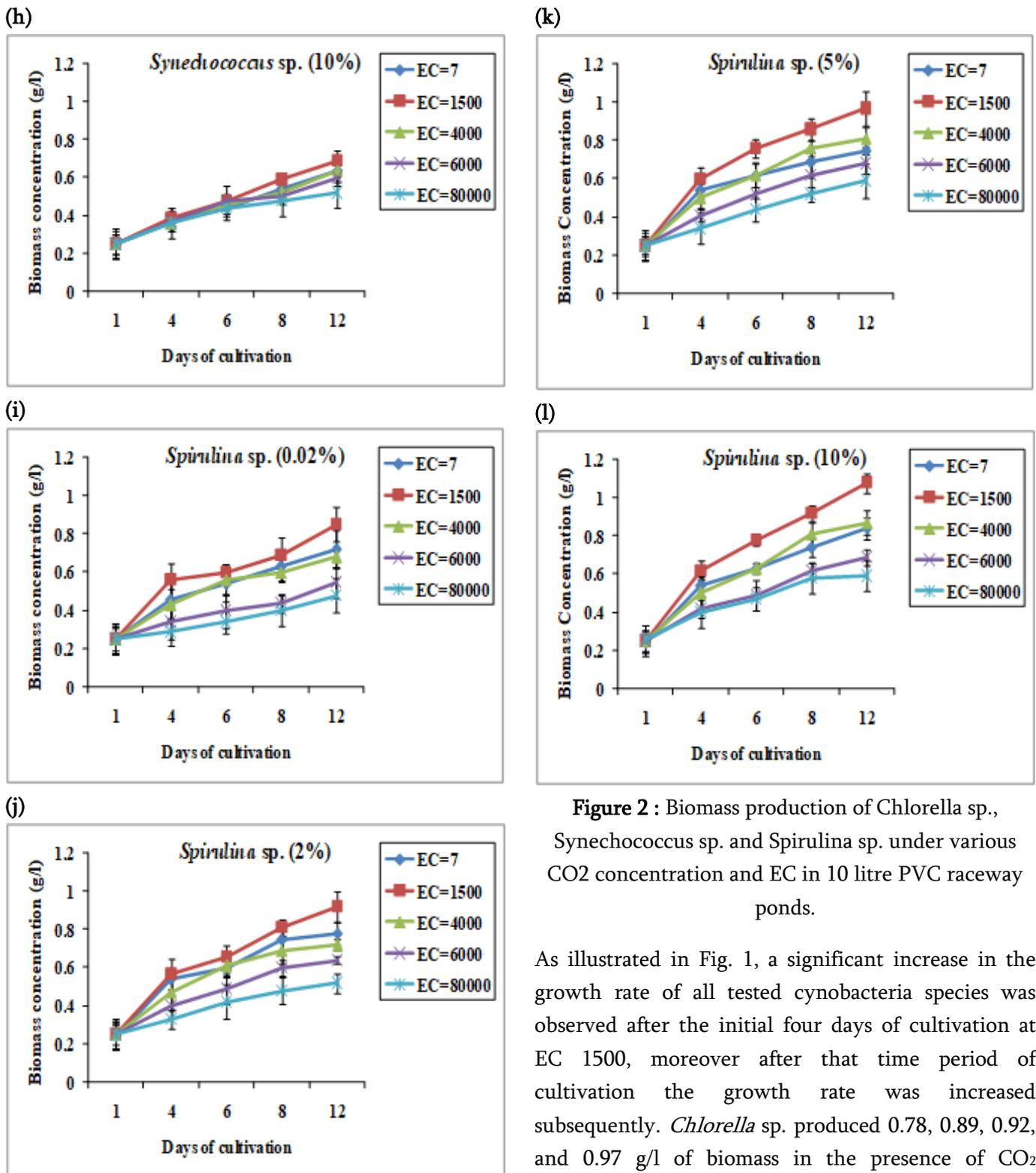
**Figure 2 :** Biomass production of *Chlorella sp.*, *Synechococcus sp.* and *Spirulina sp.* under various CO<sub>2</sub> concentration and EC in 10 litre PVC raceway ponds.
