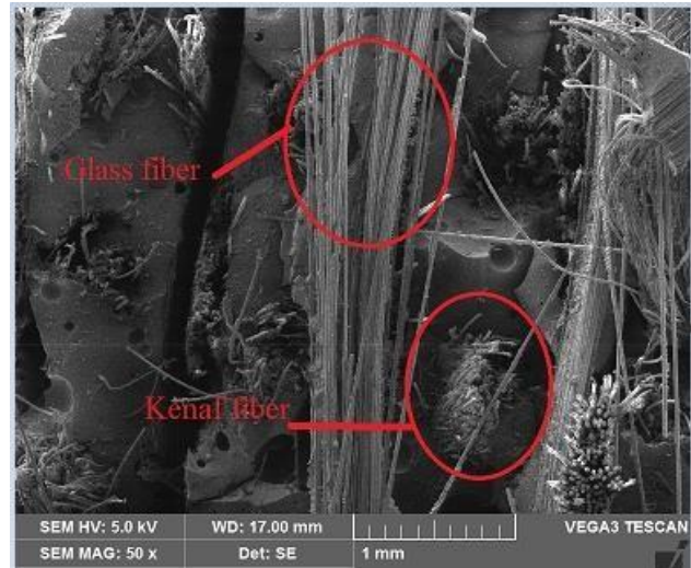
Fig: SEM images of Kenaf/Glass fiber composites
