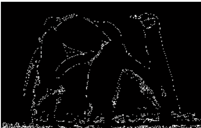
Figure 8: Canny edge detection technique used
