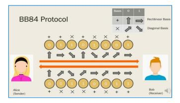
1. Alice and Bob communicate across a Quantum Channel in the first stage. Alice chooses an equal-length string of bits and bases (rectilinear or diagonal) at random.
