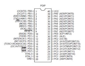
Figure 2. Pin diagram of ATMEGA162V
