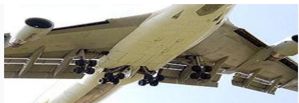
Wing and fuselage undercarriages on a Boeing 747-400, shortly before landing
