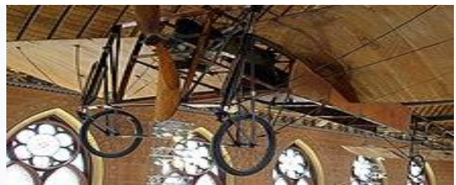
The "castoring" main gear arrangement on a Blériot XI
