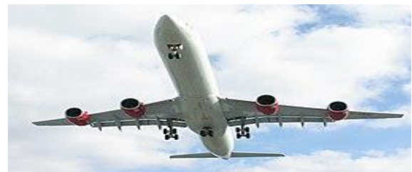
The A340-600 has an additional main undercarriage on the fuselage belly
