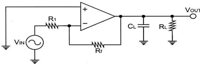
Fig. 6 : Op amp gain bandwidth configuration
