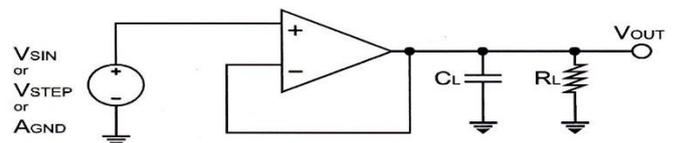
**Fig. 5 :** Op amp unit feedback configuration
