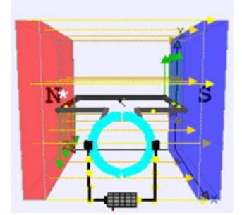
Maintenance involves regularly replacing the carbon brushes and springs which carry the electric current, as well as cleaning or replacing the commutator. These components are necessary for transferring electrical power from outside the motor to the spinning wire winding of the rotor inside the motor.
