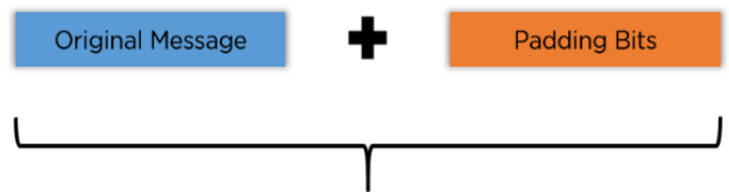
Fig 3. Total length to be 64 bits less than the multiples of 512
