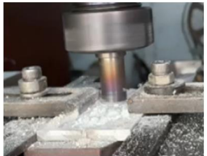
Fig.6: FSP Process with pin
