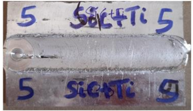
Fig.7: Friction Stir Processed Specimens
