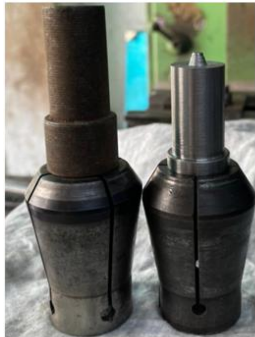
Fig.1 : FSP Tools With and without pin
