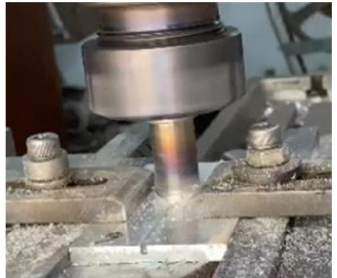
Fig.5: FSP Process without pin
