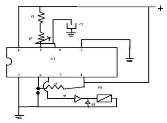
After the time is over the switch needs to be reset so that the voltage supply from the battery to the delay circuit and the to the plates will supplied continuously. The battery of 12 volt dc will be used for the delay circuit and also the power supply from the mains supply will be used. so here the 230 volt ac will converted top 12 dc pure dc and this two supply will supplied alternatively through the toggle switch that will be used for changing the power source from battery to mains.
