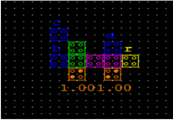
Fig. 15 QCA layout for the output R
