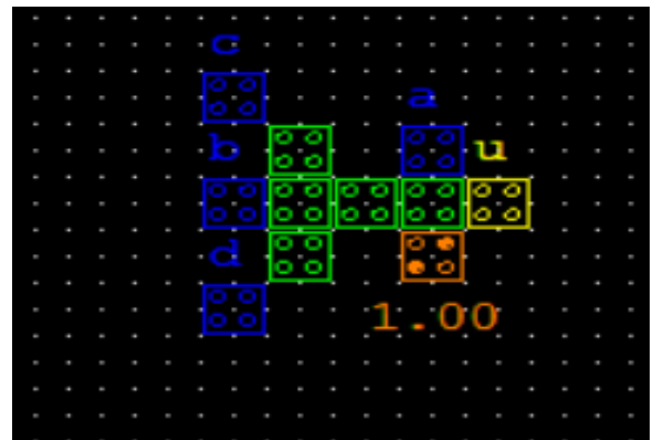
Fig. 18 QCA layout for the output U
