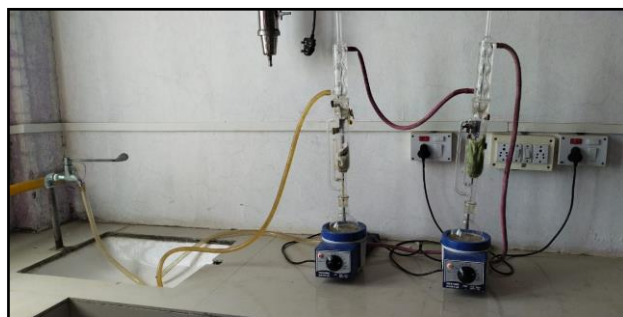
Fig.no-5 Extraction by soxhlet apparatus
