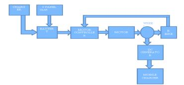
Figure 1. Block Diagram of E-BIKE
