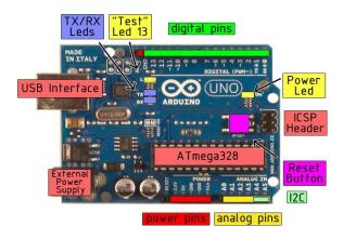
Figure 5. Arduino Uno Controller
