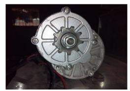
Figure 2. DC gear head Motor
