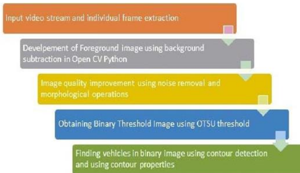
Fig 11: Systematic flow diagram of the image processing operations for obtaining the count of the present vehicles
