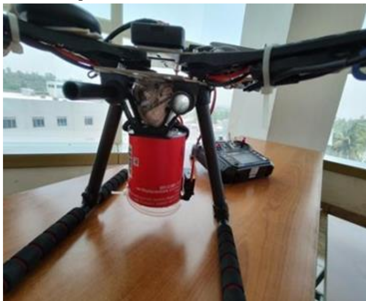
Fig.2) Fire Fighting Ball.Mounted On Drone
