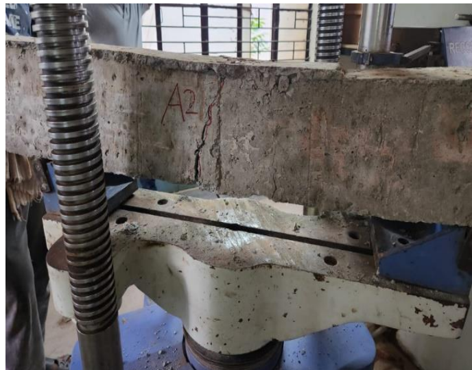
Fig. 4 Failure and cracking pattern of beams.
