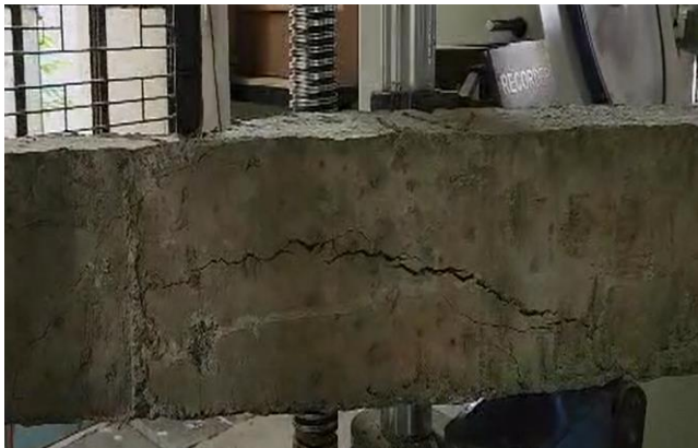
Fig. 4 Failure and cracking pattern of beams.
