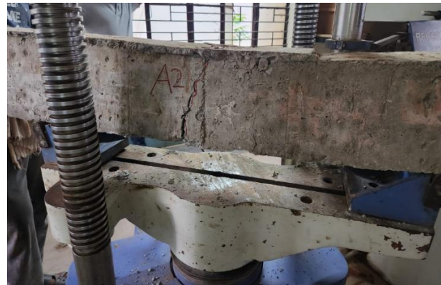
Fig. 4 Failure and cracking pattern of beams.
