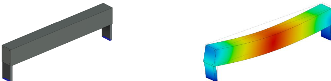
Fig.5 FE Model for concrete and Deflection Profile
