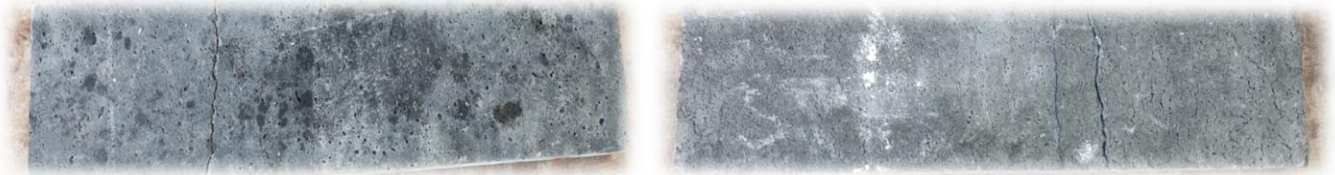
Figure 8. Rupture mechanism of designed samples under flexural loading.
