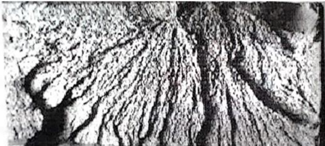
Fig 6 Radiating Ridge Fracture Surface (Callister, W.D., Page 186)
