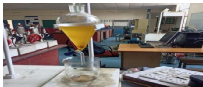
Fig.1 : Separation process of sesame biodiesel and glycerine in the funnel
