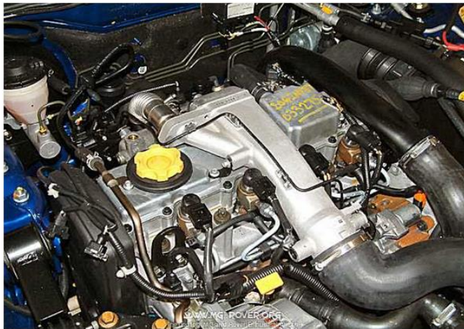
Figure 2: Actual picture of multi-cylinder C.I. research engine
