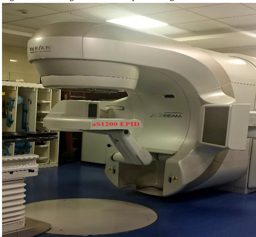
Figure 2 EPID in planned position to carry out PSQA
