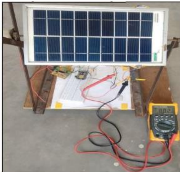
Fig. 5. Complete setup of automatic single axis solar tracker system
