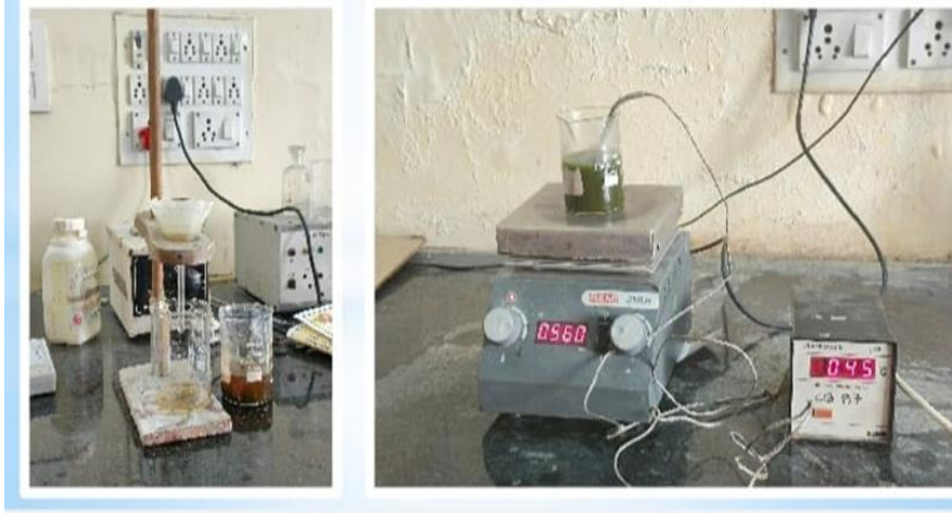
Fig. 1 Preparation set up of copper oxide nano particles
