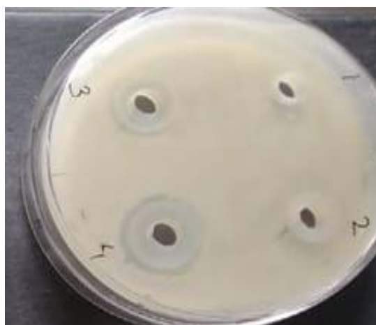
Figure- 2. Zone of inhibition observed using ZnO against different pathogens.
