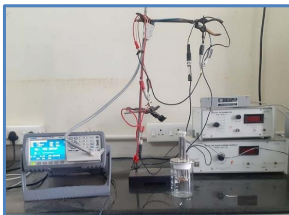
Fig.1: Experimental arrangement of \text{NiFe}_2\text{O}_4/\text{rGO} gas sensor
