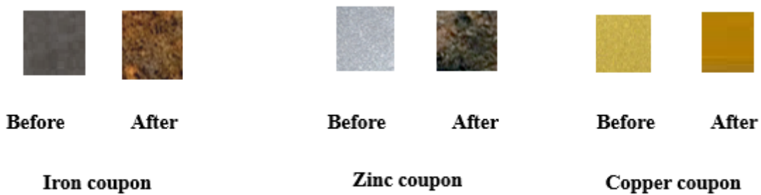
Fig 3. Appearance of Metal coupons after corrosion
