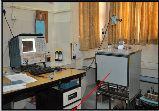
Temperature control bath with an accuracy of \pm 0.1^\circ \text{C} . Fig. 1 Experimental setup of TDR with temperature controller bath
