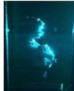
Figure 8. Photograph of Denisyuk hologram reconstructed using 488 nm laser
