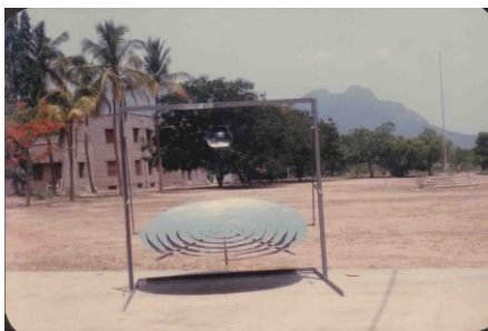
Figure 1. Concentrator with Absorber coated with smoke
