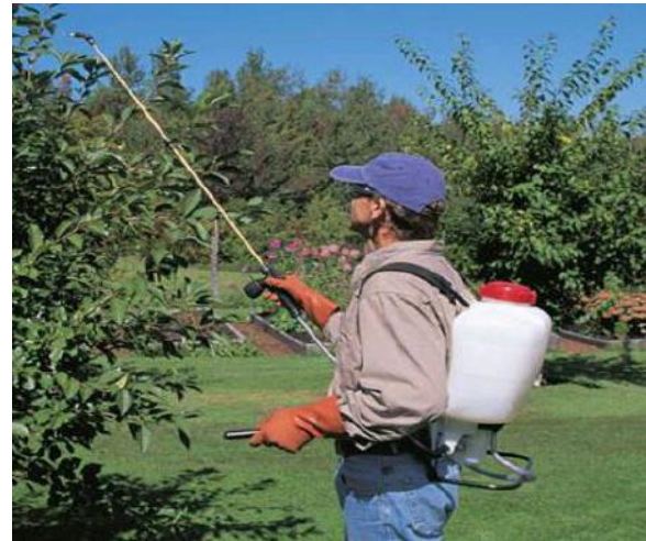
Figure 1. Backpack (knapsack) sprayer
