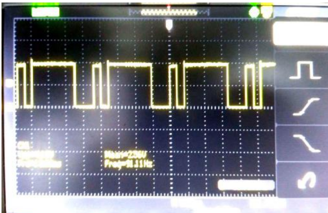
Figure 9. Output Waveform of Programmed Microcontroller IC of Pin 4
