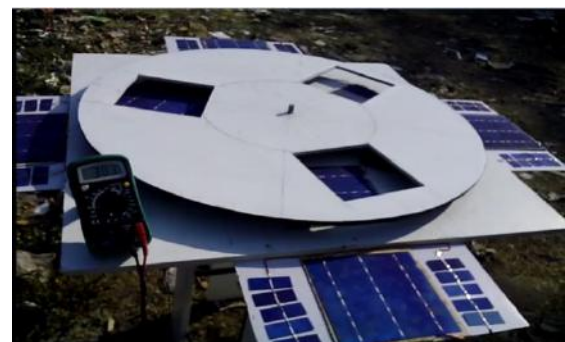
Figure: 12 Rotating disc with arrangements of solar cell
