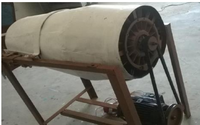
Figure 4. Fabricated Hybrid Cascade thrust Reversal Prototype
