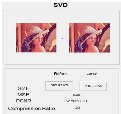
Figure 3. Compressed result using SVD
