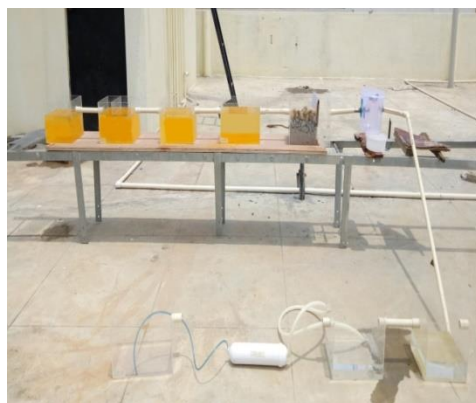
Fig. 3 Developed Effluent Treatment Plant
