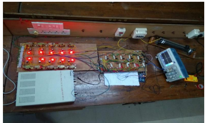
Fig. 5 Hardware setup of multilevel inverter
