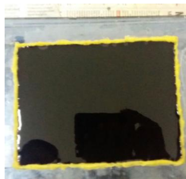
Figure 2. - Epoxy + 2g of Pbo2 + 2g of PANI
