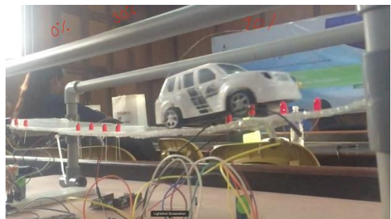
Figure 2.3. Phase 3, with 70% Deformity and cracks. The LED's light up and the Buzzer Signals Location of the vibrational Anomaly.
