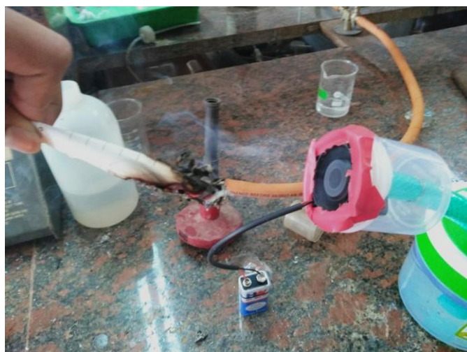
Figure 1. The air is sucked through intake fan.
