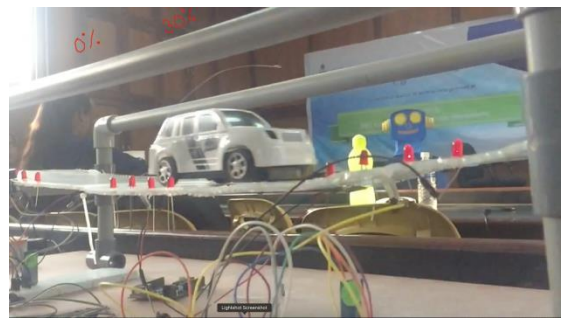
Figure 2.2: Phase 2, with 30% deformity. The presence of cracks is detected with the signal sent by the Piezo Electric Sensor. The Vibration travels to Phase 3(70% deformity) through the body of the structure. At Phase 3 The presence of increased deformity and cracks is detected even before load passes through the section. (As shown in Figure 2.3 )
