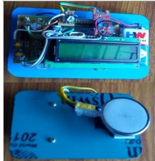
Fig 3.1. Head Display Stethoscope with Temperature Sensor
