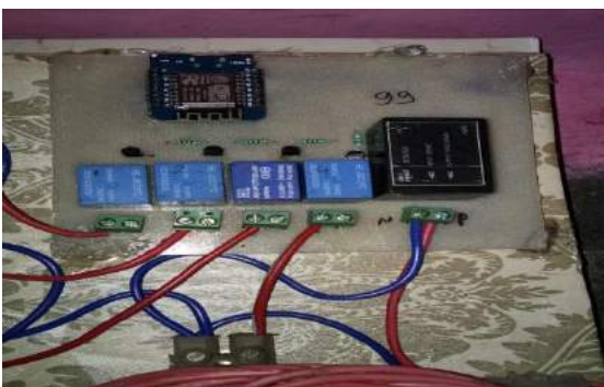
Fig: Circuit connections with 4 relays.
