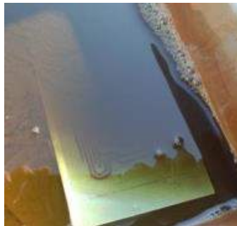
Figure 6.7.2 PCB during etching process
