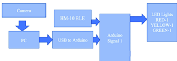
Fig (iii) Traffic density measurement using camera system [2]
