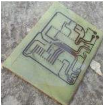
Figure 6.7.3 PCB after etching process
