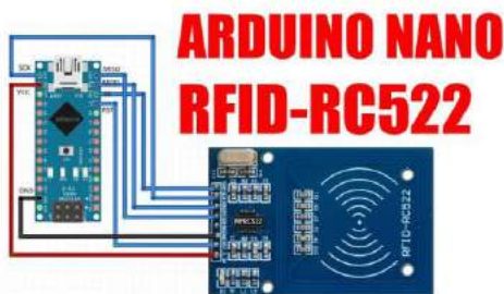
Figure 6.3 Arduino Nano to RFID
