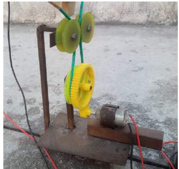
Figure 5 : Solar panel tracking using dc motor.
