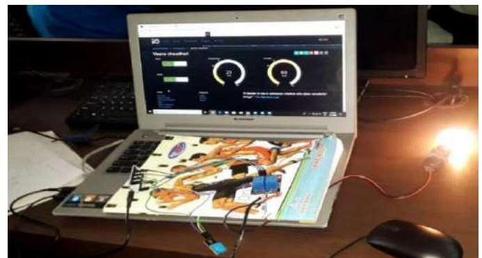
Fig 1 : IOT home automation dashboard developed on adafruit
