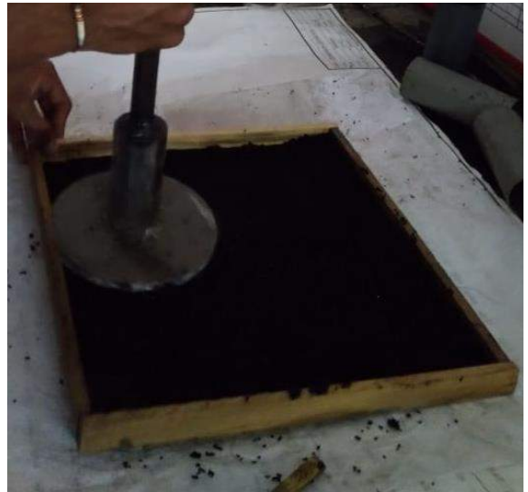
Fig.4- preparing sheet by providing compaction
