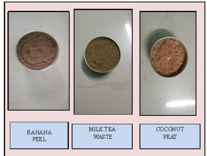
Figure 1:- Shows the dried powder of (a) Banana peel, (b) Milk tea waste (c) Coconut peat
