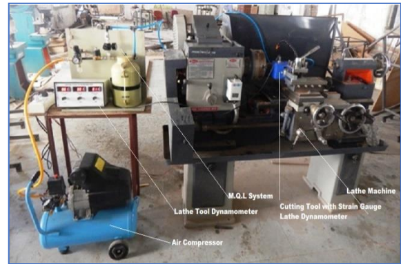
Figure 3: Experimental Set up with MQL System
