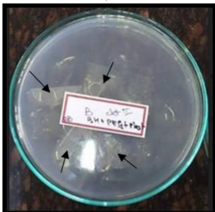
FIGURE 1 : LDPE STRIPS (INDICATED IN BLACK ARROWS) OVERLAID ONTO SOLIDIFIED BUSHNELL HAAS AGAR IN PETRI PLATE
