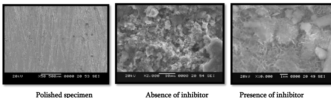
Figure-3 SEM Results of carbon steel with or without inhibitor.
