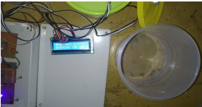
Fig.4: LCD display shows the availability of the medicine
