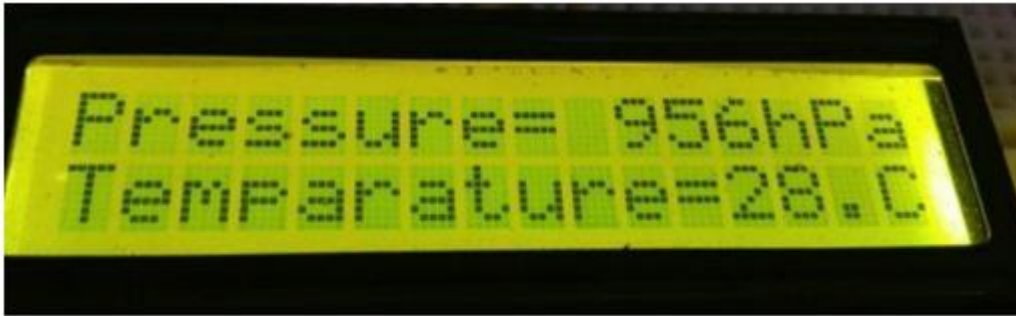
ii. LCD Shows Temperature and Pressure Levels
