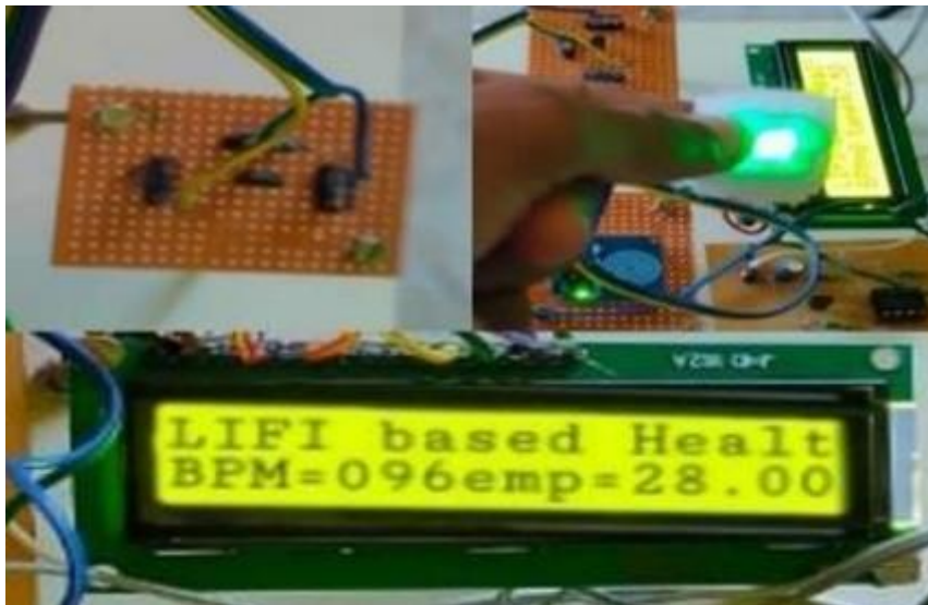
Fig. 9. Working Model of LM35 Sensor, Heart Sensor and Output
