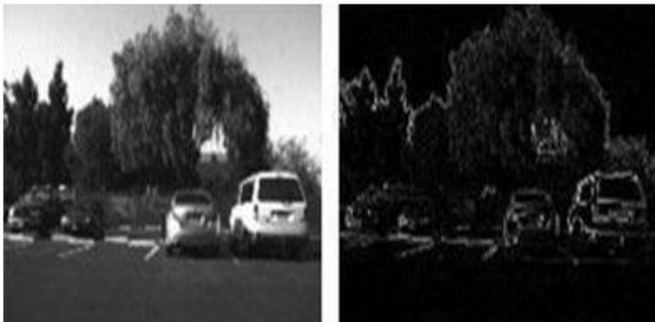
Image segmentation using the Sobel method.
