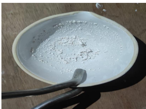
Fig. 2. Preparation of MgO nano particles by using aloe Vera leaf extract
