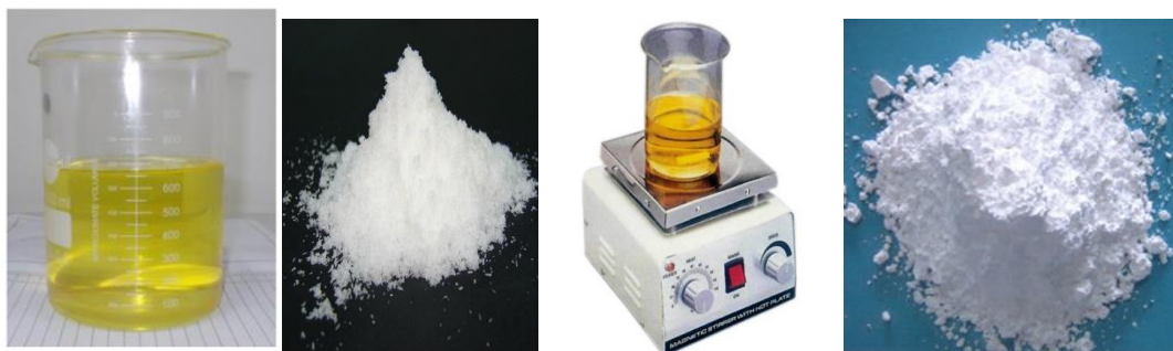
Neem Extract Magnesium Nitrate Mg(NO_3)_2 Solution heated & continuous stirring Magnesium oxide nanoparticles
